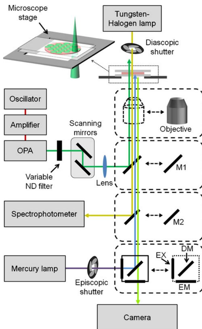
**Fig. 1** Schematic illustration of the experimental system for laser-driven adsorption of fluorescent proteins on gold nanoparticles. *M1*, *M2* broadband mirrors, *ND* neutral density, *EX* excitation filter, *EM* emission filter, *DM* dichroic mirror, *OPA* optical parametric amplifier
