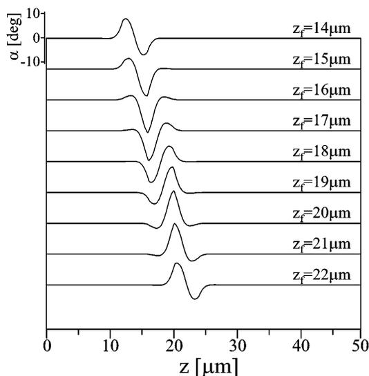
FIG. 2. The molecular reorientation induced by a focused laser beam in a LC cell. The director's angle distribution along the depth of the LC cell  $\alpha(z)$  is plotted for different depths of the focal point  $z_f$ . A linear twisted structure is formed in a periodicity of  $4 \mu\text{m}$ .
