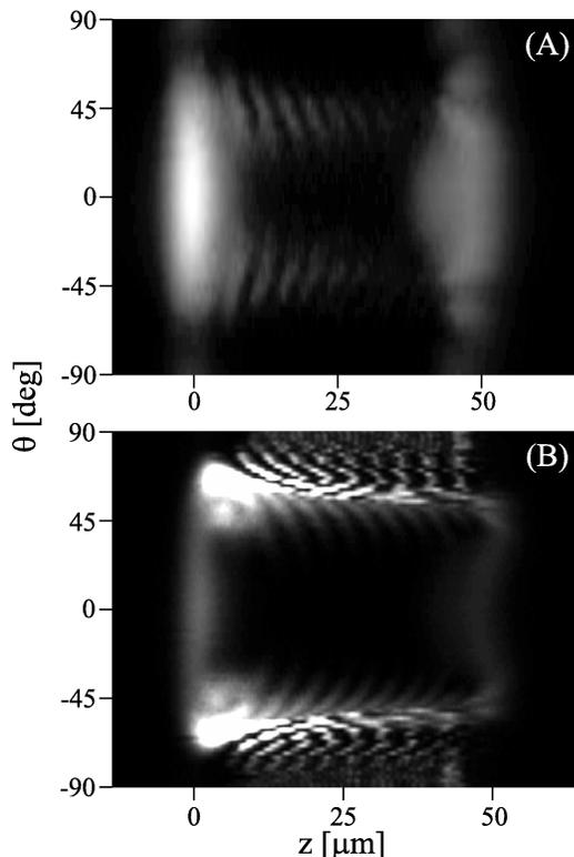
FIG. 1. THG distribution in a nematic LC cell for different linear polarization states with average laser intensity of (A) 100 mW, and (B) 200 mW. Bright gray levels represent high THG intensities. The THG from within the LC cell has an efficiency of up to  $10^{-5}$ .
